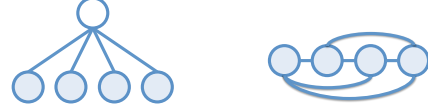
Figure 8: An MRF structure with treewidth 1, and its corresponding auxiliary MRF of treewidth n .
